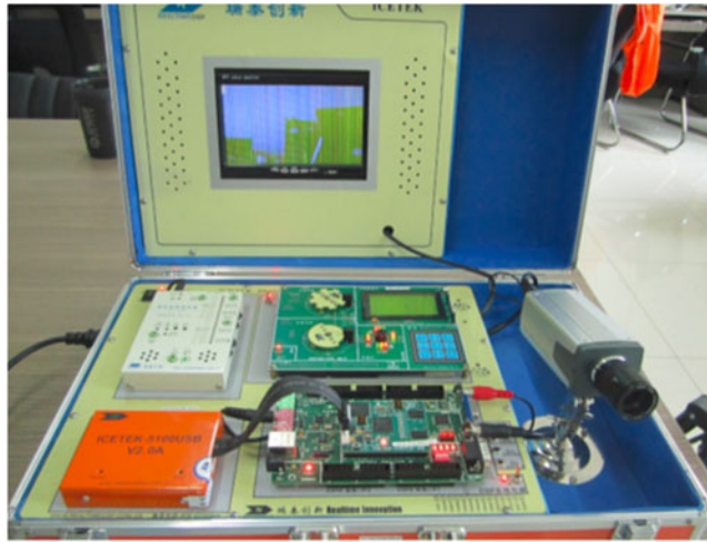
Fig. 3. Visual system used in 3D reconstruction mapping. The system is shown performing digital processing on an image captured by an RGB camera.
