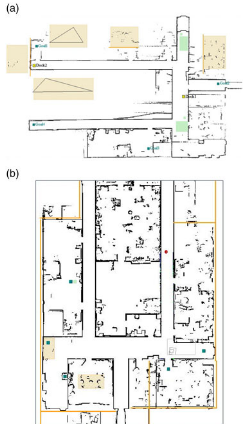
Fig. 11. New updated map produced from continuous SLAM process. (a) OOIs located and marked on new map. (b) Current original metric map updated online by the produced new map, which is corresponding to the actual current SAR environmental map.
