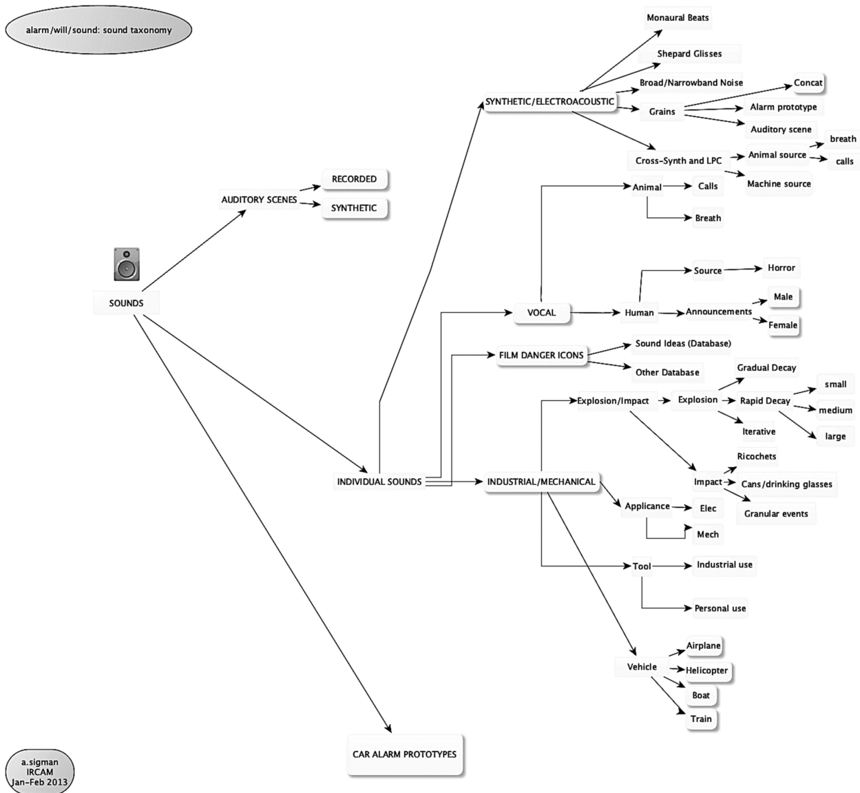
Figure 1. Alarm sound catalogue taxonomy, constructed in January–February 2013. ‘Elec’ and ‘Mech’ (under INDUSTRIAL/MECHANICAL→electrically powered and mechanical sources, respectively). ‘Concat’ (under SYNTHETIC/ELECTROACOUSTIC→Grains) refers to the concatenative synthesis technique by which the entries in this sub-category were generated.
