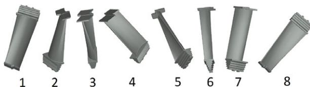
**Figure 7.** Eight images needed to be taken from different angles of the turbine blade for the sake of inspection.
