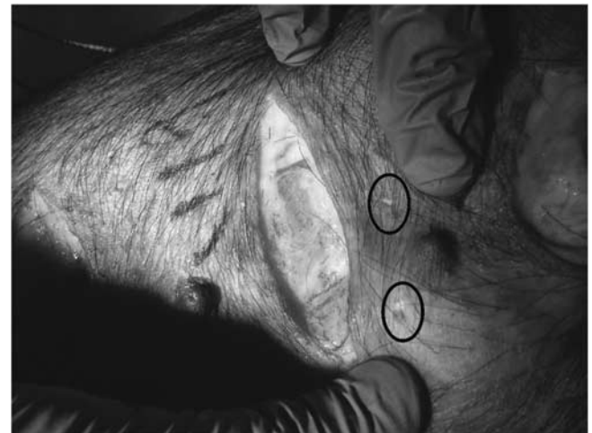
Figure 9. Minor Skin Tear Seen on the Encompassed Device Parallel Pull from Swine Model.
