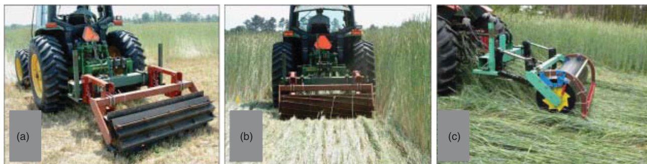
Figure 1. Different roller types: (a) original Brazilian type straight bar roller, (b) curved bar roller-crimper and (c) smooth roller with crimping bar (U.S. patent no. 7,604,067 B1).
