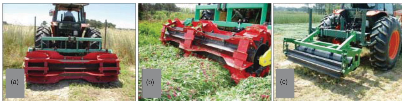
Figure 2. (a) Roller-crimper for elevated beds: one row and two furrows. (b) Roller for elevated beds: two rows and three furrows. (c) Two-stage roller/crimper designed to operate with smaller tractors (40 HP power source). The roller comprises a 30 cm diameter smooth drum which rolls down the cover crop and second small 15 cm diameter roller with six equally spaced 0.6 cm-thick crimping bars on the drum's perimeter. Depending on cover crop type and amount, crimping force can be adjusted by changing preloading force of two adjusting springs to obtain the best crimping characteristics for a particular cover crop. Patent pending—U.S. Patent no. 7,562,517 B1.
