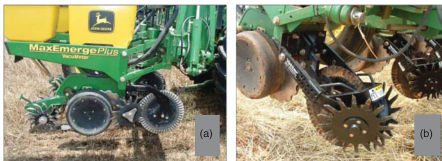
Figure 3. (a) John Deere no-till planter for planting cotton seeds into rye residue cover using DAWN™ row cleaners and (b) John Deere no-till planter with attached Yetter™ row cleaners.
