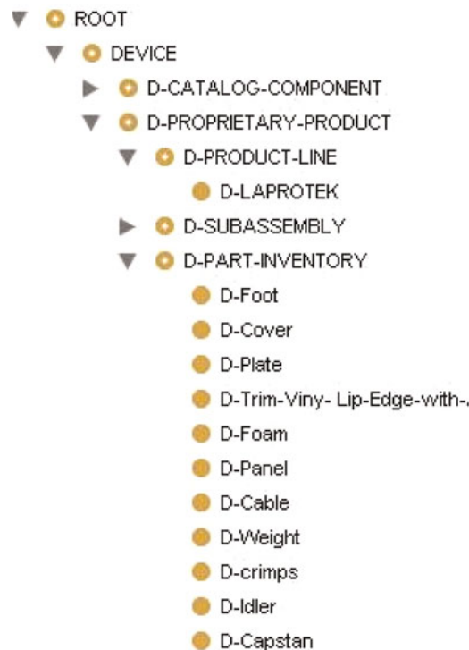
Fig. 8. Part of the device taxonomy for the surgical robot design. [A color version of this figure can be viewed online at journals.cambridge.org/aie ]
