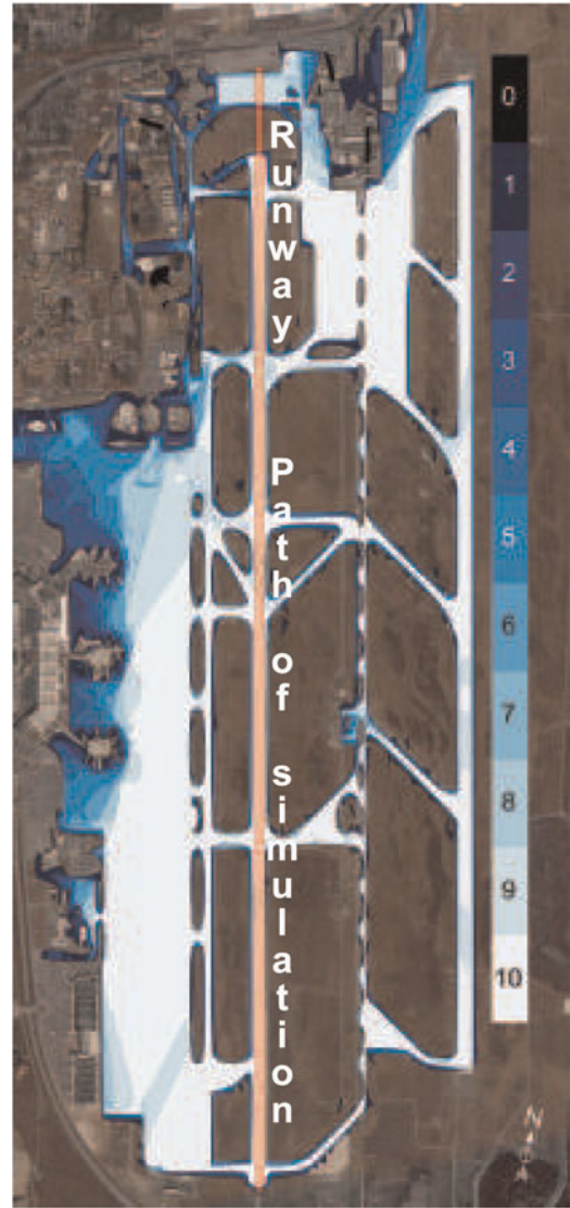
Fig. 1. Number of visible stations from each point of the airport (the line shows the path used in the simulations).
