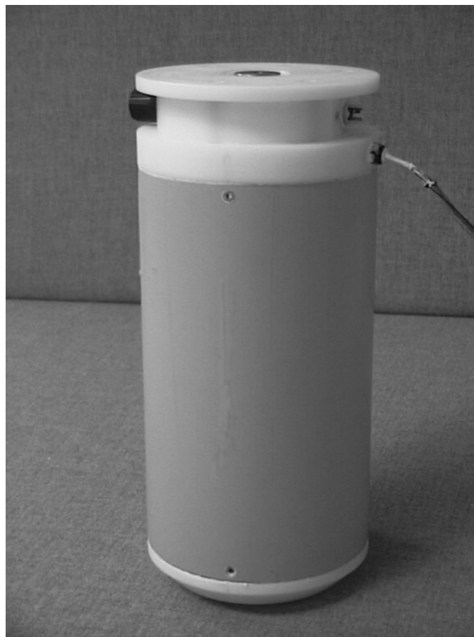
Fig. 3. DIVEBOT. (Length: 38 cm, Diameter: 16.8 cm, Weight: 8.4 Kg).
