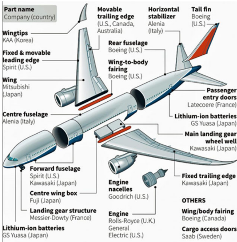
Figure 2. 787 Dreamliner structure suppliers – selected component and system suppliers
