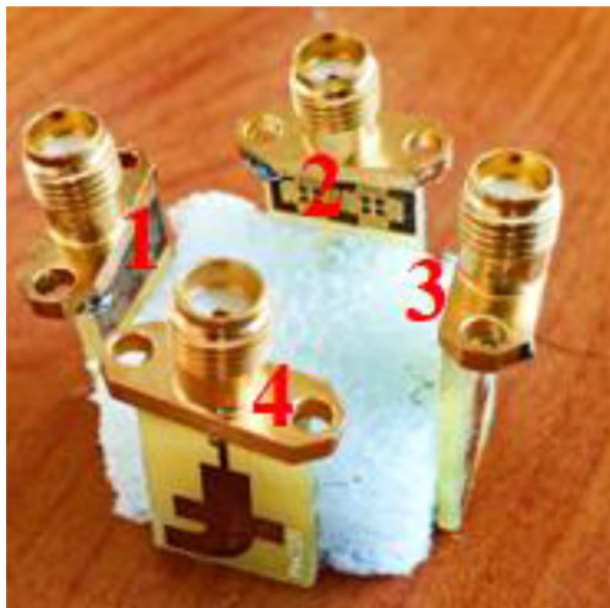
Fig. 4. Fabricated prototype for the proposed four-port UWB-MIMO antenna.
