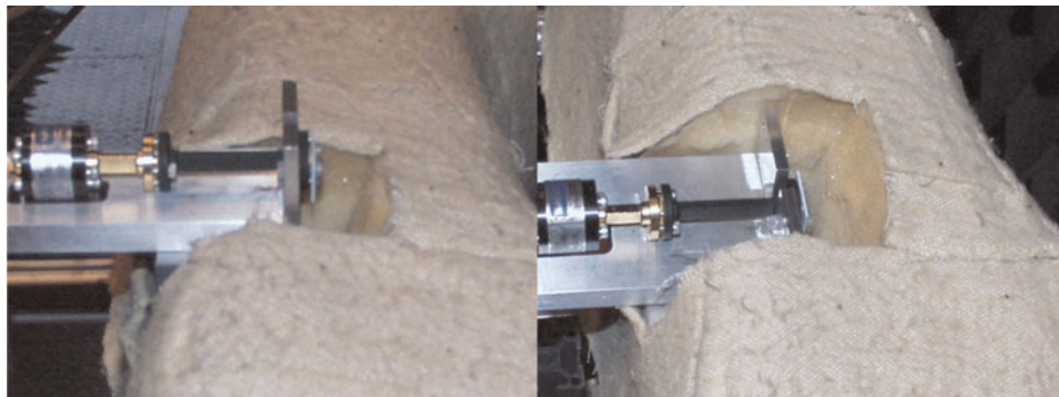
Fig. 6. Different position of the antenna relative to the seat cover: top of the foam (left side) and inside the foam (right side).
