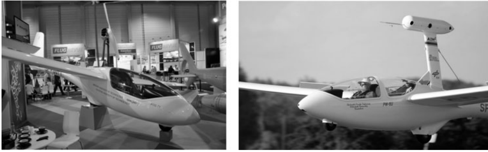
Figure 4. Electric glider AOS-71 (left) and the unpowered glider PW-6U with dorsal camera pod (right).
