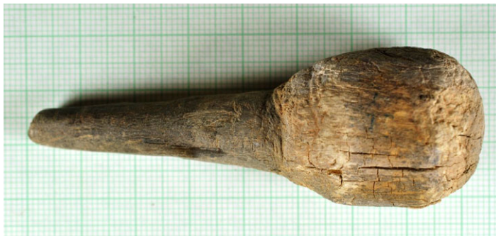
Figure 2 Photograph of the bunt in which we observed large CO 2 pressure rises during Ar-plasmas. Notice the cracks and high porosity permitting the inclusion of considerable water into the interior of the artifact. The smallest graph paper squares are 0.1 cm.
