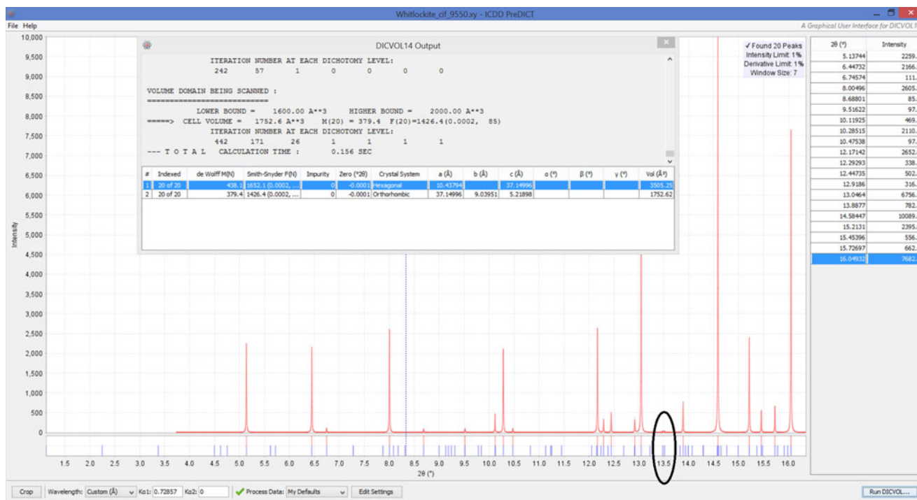
Figure 3. (Colour online) After a successful DICVOL14 run : (i) a list of suggested unit cells is displayed with minimal information. (ii) Once a specific solution is selected (highlighted), all the related calculated Bragg peak positions are graphically displayed (blue marks) below the peaks used for the indexing. In good cases such as the one shown in the figure, Bragg peaks not selected for indexing will now become accounted for (black oval).
