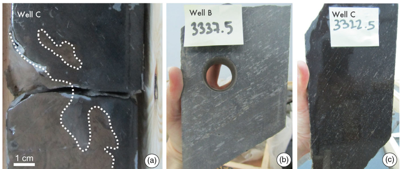
Fig. 7. (a) Hardground in light brown carbonates; the core sample is approximately 10 cm wide. (b, c) Pervasive presence of crinoids (recognized as the light-coloured particles) in Well B and Well C. The stickers indicate the depth of the core sample. Note that the bedding is oblique to the long axis of the core.
