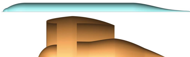
Figure 3. The podded configuration serves as a reference and models fuselage (top) and propulsor (bottom) separately.
