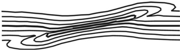
Figure 9. A sheath/intrafolial fold produced by pronounced top-to-right shear on the CE of a flanking structure. Reproduced with permission from Exner, U. & Dabrowski, M. 2010. Monoclinic and triclinic 3D flanking structures around elliptical cracks. Journal of Structural Geology 32 , 2009–2021, Elsevier.
