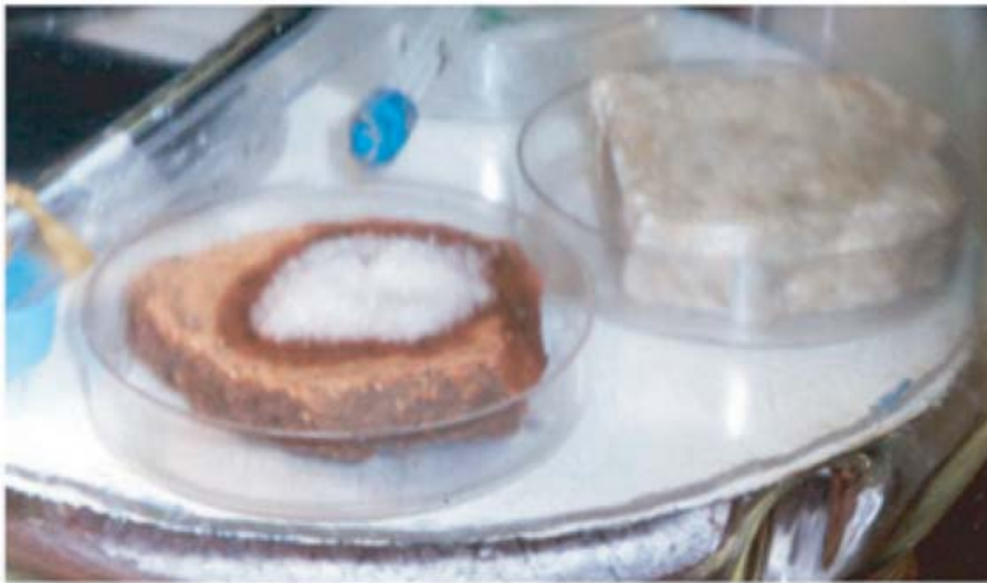
Fig. 13. Mars in a jar: liquid water from frost on rock under Martian conditions. Courtesy of D. Gan and L. Kuznetz, University of California, Berkley.
