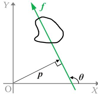
Fig. 1. Representation of a wrench on XY plane.
