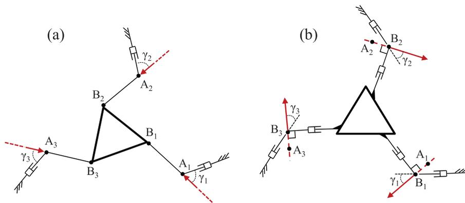
Fig. 6. 3-DOF PPMs with P actuated legs of (a) A 3-PRR PPM. (b) A 3-PRP PPM.
