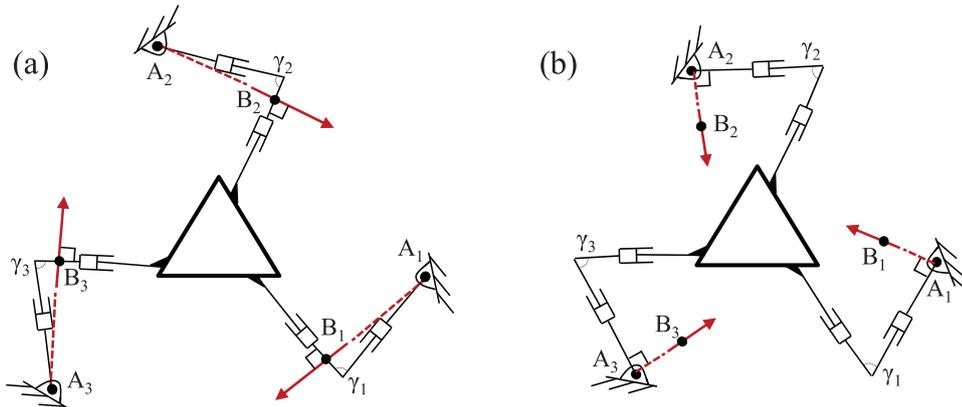
Fig. 7. 3-DOF PPMs with P actuated legs of (a) A 3-RPP PPM. (b) A 3-RPP PPM.
