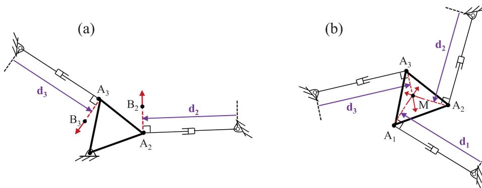
Fig. 8. Possible singularity configurations of a 3-RPR PPM. (a) Type-I singularity. (b) Type-II singularity.
