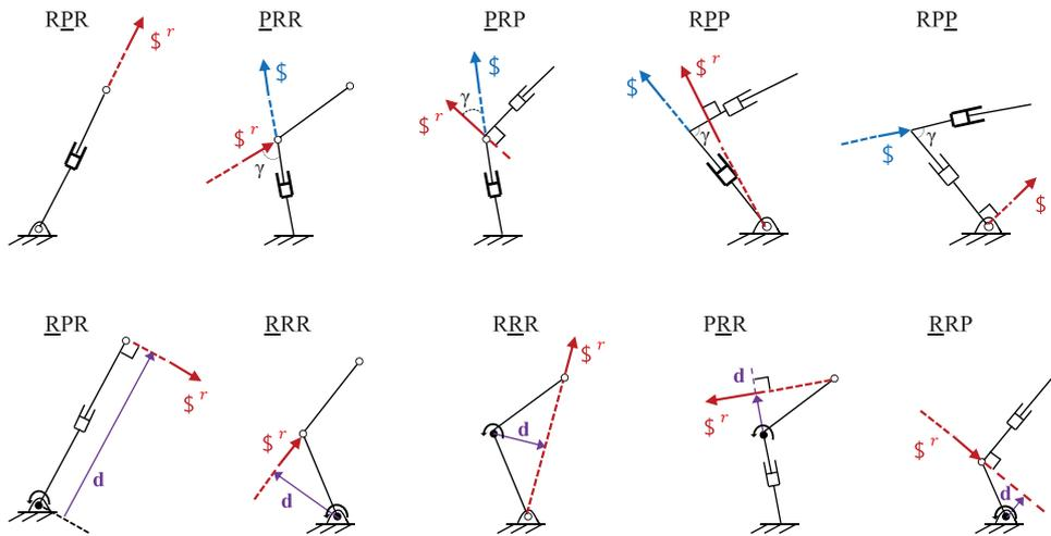
Fig. 4. Reciprocal wrenches of ten different types of legs. The underlines denote the actuated joints.
