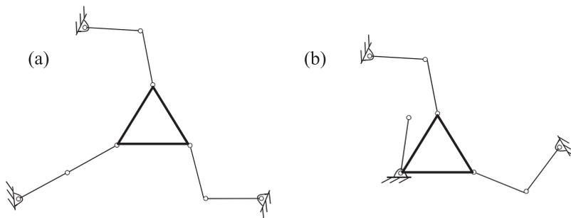
Fig. 9. Two different configurations of Type-1 singularity for 3-RRR and 3-RRR PPMs. (a) A leg is fully extended. (b) A leg is folded.
