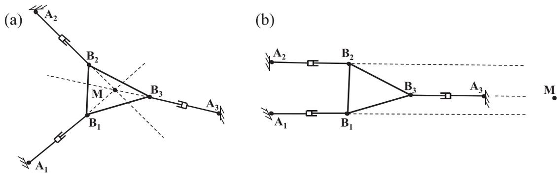
Fig. 5. The Type-II singular configurations of a 3-RPR PPM. (a) Three legs are concurrent. (b) Three legs are parallel.
