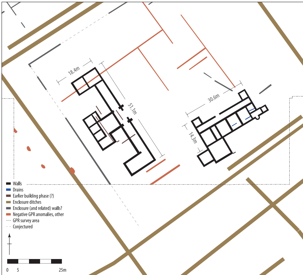
FIG. 6. Schematic and simplified interpretation of the GPR and gradiometry survey results of the Bourne Park high-status structural complex. ( Lacey Wallace and Lieven Verdonck )
