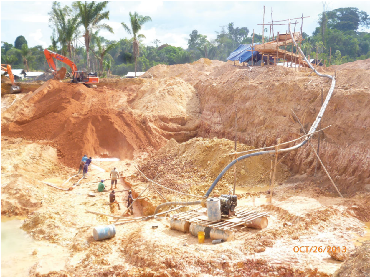
Fig. 6. Mechanical hydraulic mining ('soigi spoiti') operation at Koemboekreek, south of Rosebel concession (photo: R. Finkie).
