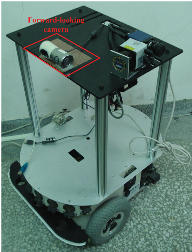
Fig. 8. (Colour online) U-BOT and the mounted forward-looking camera.
