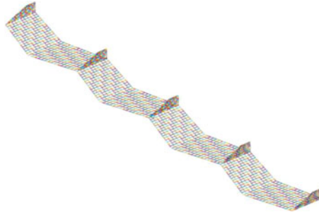
Figure 7. VLM mesh for a sample UAV design for N = 4 .
