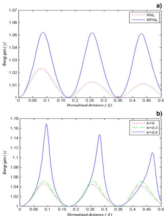
**Fig. 5.** (a) Variation of energy gain ( $\gamma$ ) by the electron with normalized distance of propagation ( $\xi$ ) for  $a = b = 0.5$ . (b) Variation of energy gain ( $\gamma$ ) by the electron with normalized distance of propagation ( $\xi$ ) for different values of decentered parameter ( $b$ ) with constant value of intensity parameter ( $a$ ), when relativistic-ponderomotive nonlinearity is operative.
