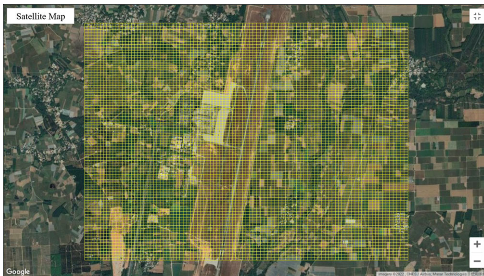
Figure 2. Spatial grid discretisation within radar surveillance airspace.
