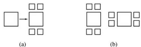
Fig. 16. A rule with LHS symmetry of D_4 and overall symmetry of D_2 (a), and the two possible ways to apply the rule to a square (b).
