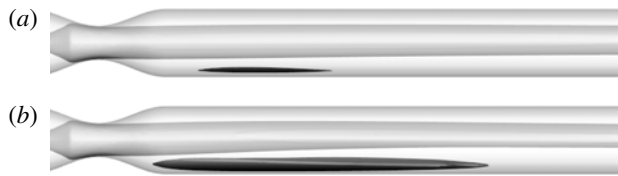
FIGURE 7. Two isosurfaces of axial velocity ( u/U = -0.5 and 2.0 ) for the flow at Reynolds number Re = 350 and eccentricity E = 0.0025 . (a) The weakly skewed solution, obtained from rest, and (b) the more strongly skewed, obtained by initializing the flow with a solution from a larger eccentricity.
