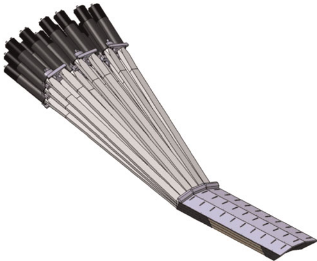
Fig. 3. (Color online) Prototype of a neutron detector under development at IPN Orsay, from (Bettane, 2010). There are three layers of plastic scintillator detectors, each 3 cm thick. The final version will cover 360^\circ in \Phi , with a bore of 60 cm.
