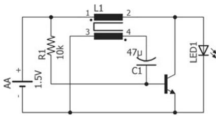
**Fig. 1.** Circuit diagram of a Joule thief: the flashing LED provides enough light to preserve *Euglena gracilis* cells in the state of dormancy while only drawing a minute amount of power from the battery.
