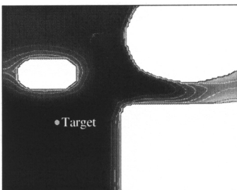
Fig. 16. 2D danger map towards the target; equipotentials give grey scale showing the minimum danger of the available trajectories; danger towards the target from points not on the road are fixed at maximum.
