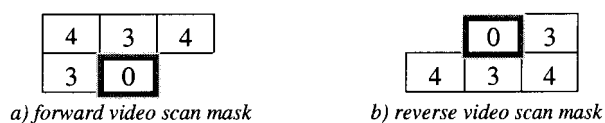
Fig. 7. Video-scan masks used in the sequential algorithm to compute the map of distances between nearest obstacle and point considered; highlighted box indicates the application point.
