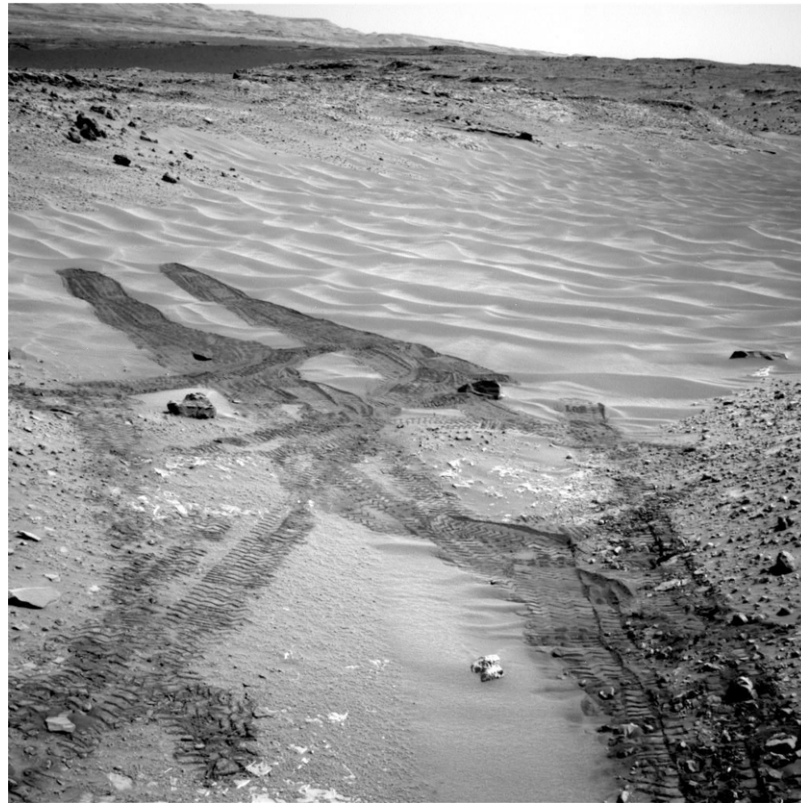
Fig. 1. The Hidden Valley on Mars ©NASA/JPL-Caltech. Curiosity experienced excessive wheel slip here and failed to traverse this region although it is relatively flat. At the beginning of the mission, Curiosity was commanded to travel on the flat surface and avoid obstacles such as rocks; however, wheel slip occurred owing to loose sand with megaripples. Wheel traces on these megaripples indicated that Curiosity gave up traversing this surface and turned back to avoid getting stuck.
