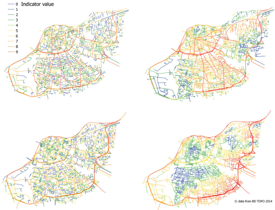
Fig. 12. Maps of the four centralities restricted on sample S2, after being computed on S4. Upper right: the betweenness computed on the dual space (ways). Upper left: the structrality computed on the ways. Lower left: the betweenness computed on the arcs (normal space). Lower right: the closeness (equivalent to the structrality computed on the arcs). The four results are different, but there are some similarities: the betweenness are very contrasted, with high betweenness being next to a very low one, on a noisy background, while the structralities, being the result of a mean distance measure, are by nature continuous and more diffuse. In the same time, the betweenness and structrality on the ways reveal some similar underlying structure, with converging axes toward the historical center of Avignon, while the ones computed on the arcs reveal more the peripheral ways. (Color online)
