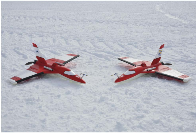
Fig. 1. Small Unmanned Meteorological Observer (SUMO) unmanned aerial vehicles (UAVs) at Williams Field, Antarctica.
