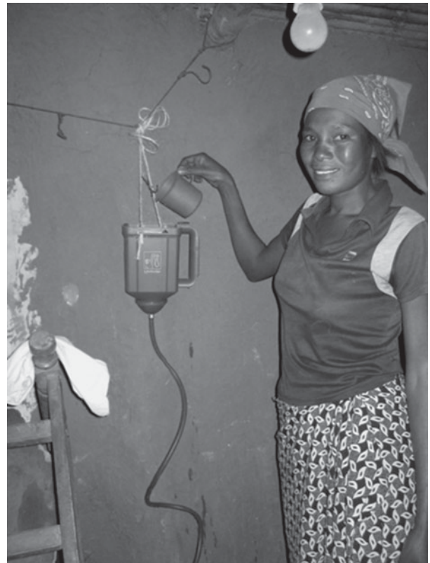
Fig. 2. Domestic water filtration device (Life Straw, Vestergard Frandsen) in use in Lusaka. This filtration unit contains a pre-filter to remove larger particulates and a textile filter to remove microbe contaminants with an effective pore size of 20 nm. The unit is expected to last for 3 years with a daily load of 16 litres.
