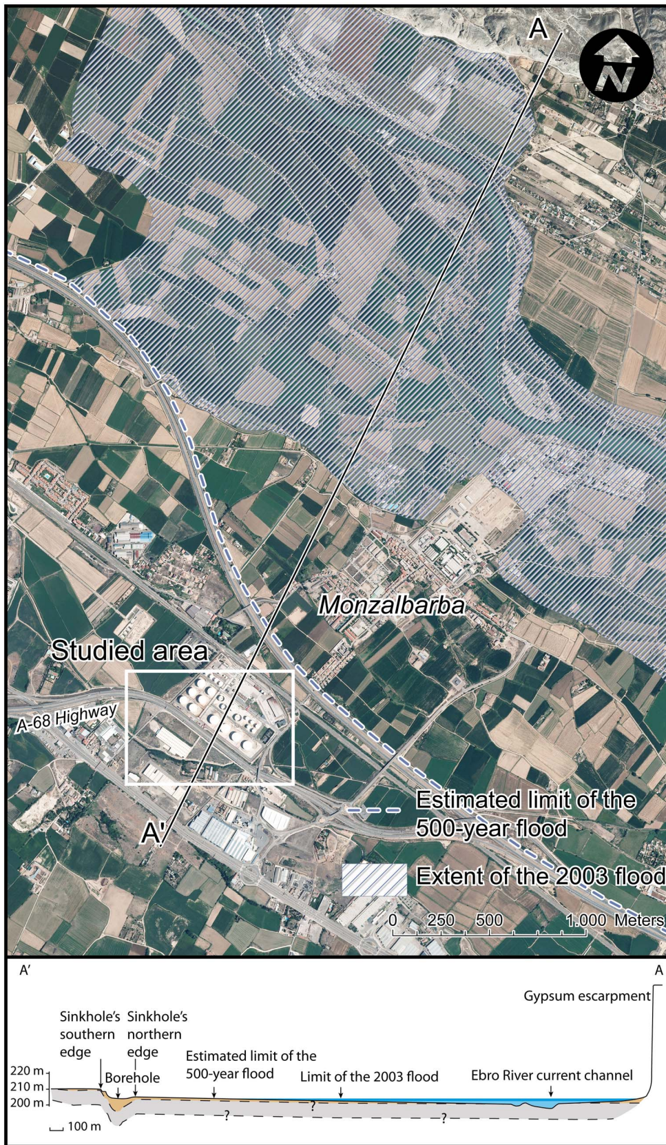
Figure 2. (color online) Orthoimage from 2002 and topographic profile showing the location of the studied sinkhole, the area covered by the 2003 flood, and the estimated limit of the 500 yr flood, according to the Ebro River Basin Water Authority.
