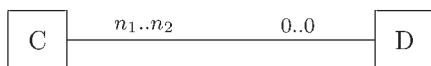
Fig. 4. A binary association modeling a conflict between the two classes, C and D , via a 0..0 multiplicity.
