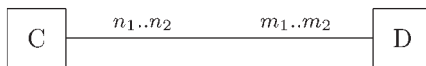
Fig. 1. Two classes, C and D , a binary association between them, and multiplicities restricting the number of allowed links.
