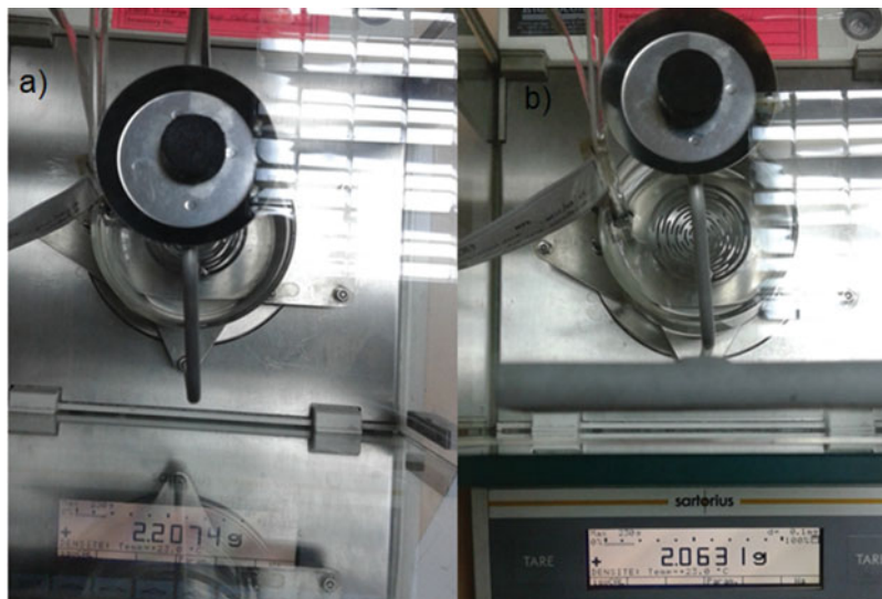
Figure 10. (Colour online) Measuring the weight of specimen; (a) before the abrasion test; (b) after the abrasion test.
