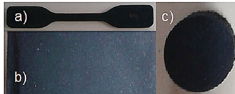
Figure 2. (Colour online) Standard shape types for tyre specimens; (a) Dumbbell shape; (b) Rectangular; (c) Circular shape.
