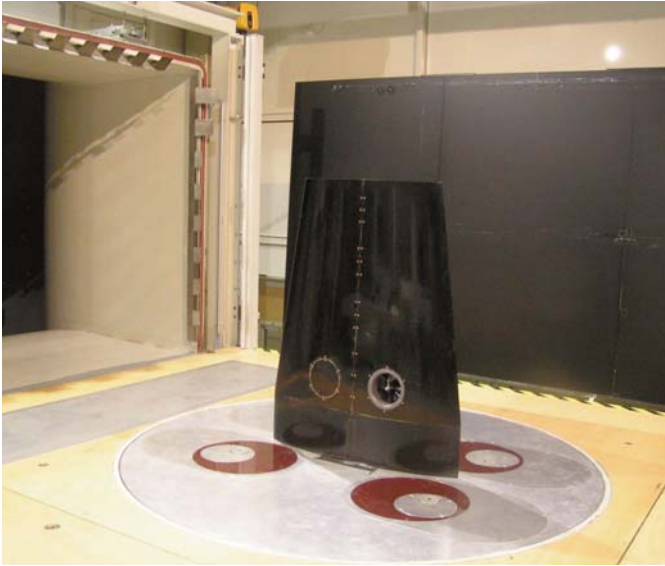
Figure 2. Fan-at-rear configuration in wind tunnel.
