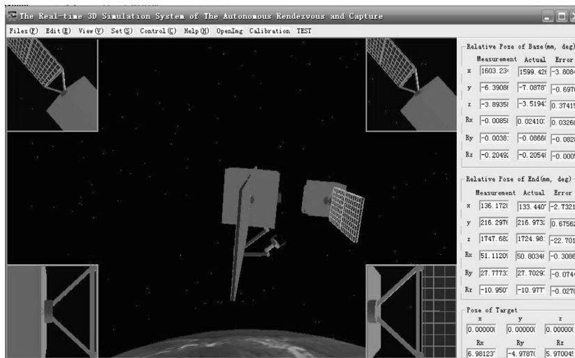
Fig. 21. The chaser reaches at the desired pose and the manipulator is commanded at t = 68.25 s.
