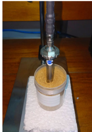
Fig. 7. Dielectric parameter measurement of dried banana leaves to powder using a dielectric probe technique.
