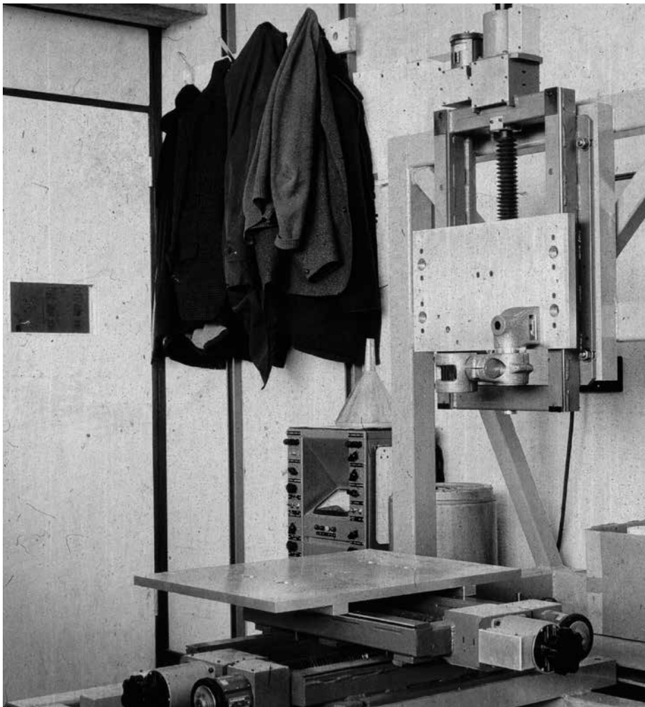
4 The Cambridge CAD Group's model-making machine was an early 5-axis CNC machine inspired by Bezier's UNISURF system, February 1971.
