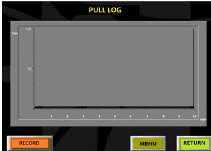
Figure 10. Screen providing data on pulling force during manoeuvres. This information will be stored in the system's memory (Carral Couce et al., 2011).
