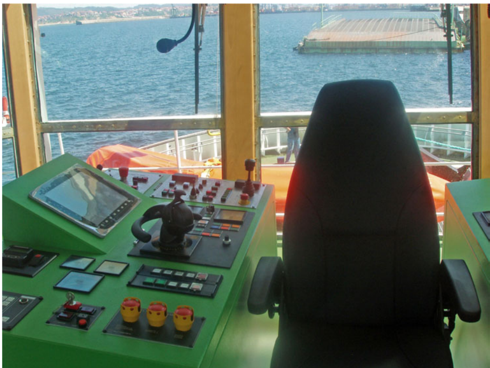
Figure 13. Control panel with touch screen on the top for manoeuvring control in a tug with azimuthal propulsion.
