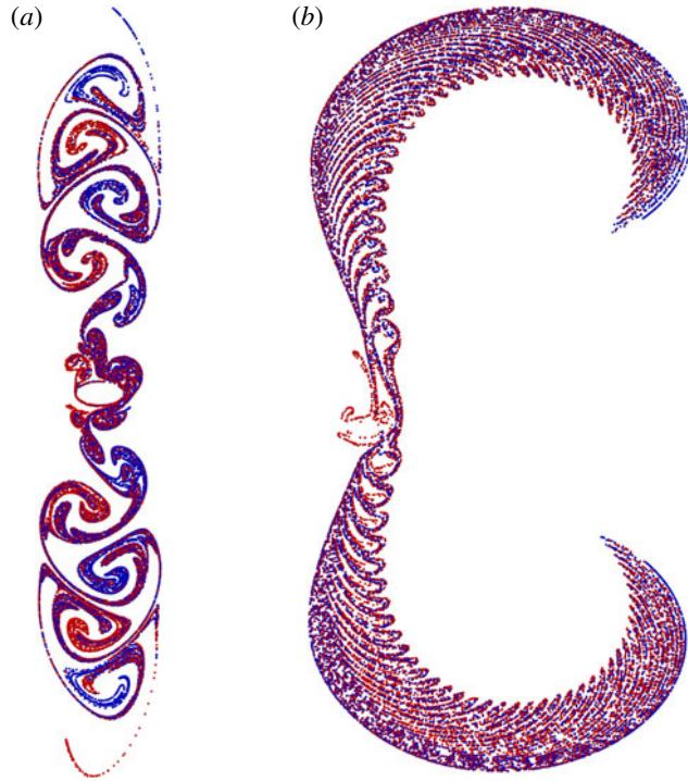
FIGURE 7. Computed positions of massless particles advected from close to the elliptical foil with AR = 0.5 in flows with parameters (a) KC = 4.89 , \beta = 19 ( QP_H -type asymmetry) after a release during the interval [130T_0, 150T_0] ; and (b) KC = 8.16 , \beta = 5 (S-type asymmetry) after a release during the interval [130T_0, 170T_0] following the start of pure oscillation with period T_0 . Blue particles are released continuously from the right of the equator of the circle, and red particles are released continuously from the left of the equator of the circle.
