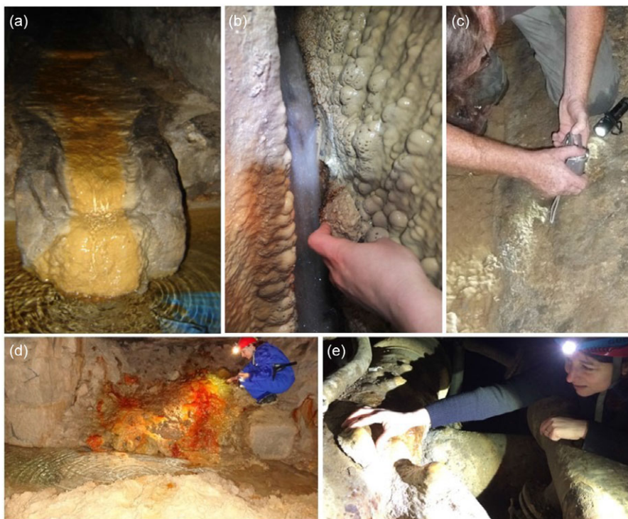
Figure 2 Pictures of the studied sites: (a) historical fountain of Saint Martin Manhole with \text{CaCO}_3 crust (sample SM B); (b) Rungis aqueduct, south of Paris, with sample Run1 at the time of its collection in a water inlet; (c) Belleville aqueduct in northern Paris, and Bel 1 sample at the time of its collection; (d) Brasserie former quarry, with the red carbonate crust sampled (Bra 1 sample); (e) under the Neptune basin, Versailles Palace Gardens, Nep 2 sample, deposited on a pipe, by the fountain and basin leakages. (Please see online version for color figures.)
