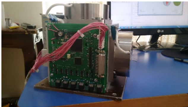
Figure 6. K. N. Toosi IMU FOG gyroscopes and Q-FLEX accelerometers (Rahimi et al., 2020), with details in Table 1.
