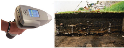
NIR (Near Infrared) gun – the 4engr company's Phazir handheld material analyser. This kind of instrument has been used in Sweden to detect bone, textile and Vitamin C (e.g. from fruit) in sections. Sources: gun: http://www.4engr.com/product/catalog/12415/index1.html ; section: editor.
