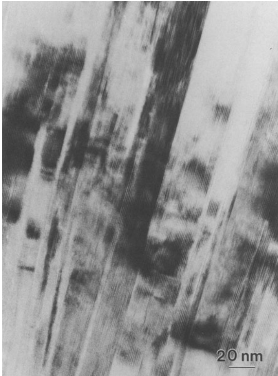
Figure 2. TEM image of chlorite showing lath-like domains.
