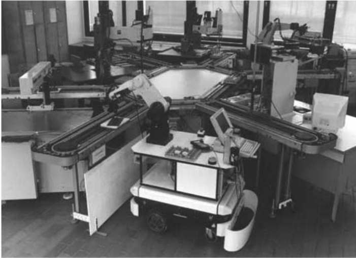
Figure 5. Holonic assembly cell consisting of 4 robots, 1 mobile manipulator connected by a pallet transport system, and working holonically together to assemble a variety of products.
