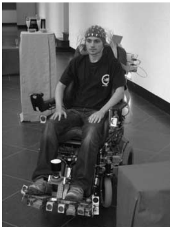
Figure 4. Intelligent wheelchair controlled by a brain computer interface (BCI).
