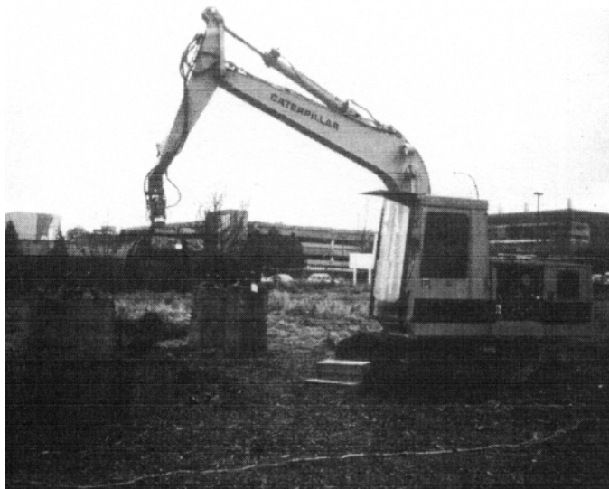
Fig. 1. Typical mobile manipulator; a Caterpillar 215B excavator-based log-loader.
