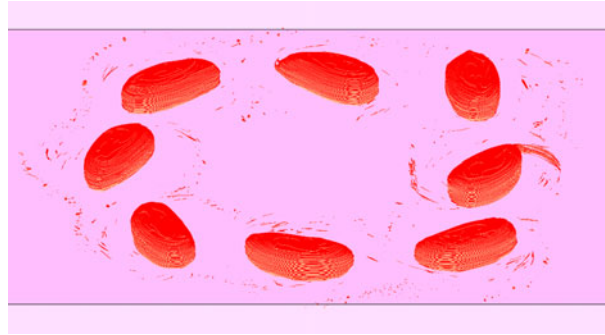
FIGURE 13. (Colour online) Orthographic view of the PV field at an angle of 60^\circ from the vertical for the torus with R_0/r_0 = 12 at t = 92 .
